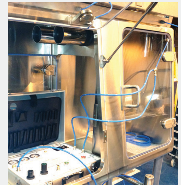
Portable rapid cycle testing at Sealing Projex or at the clients premises
